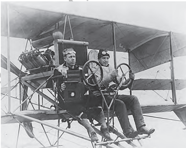
FIGURE 1.2. Early aerial photography by the U.S. Navy, 1914. This photograph illustrates difficulties encountered in early efforts to match the camera with the airplane—neither is well-suited for use with the other. From U.S. Navy, National Archives and Records Administration, ARC 295605.
