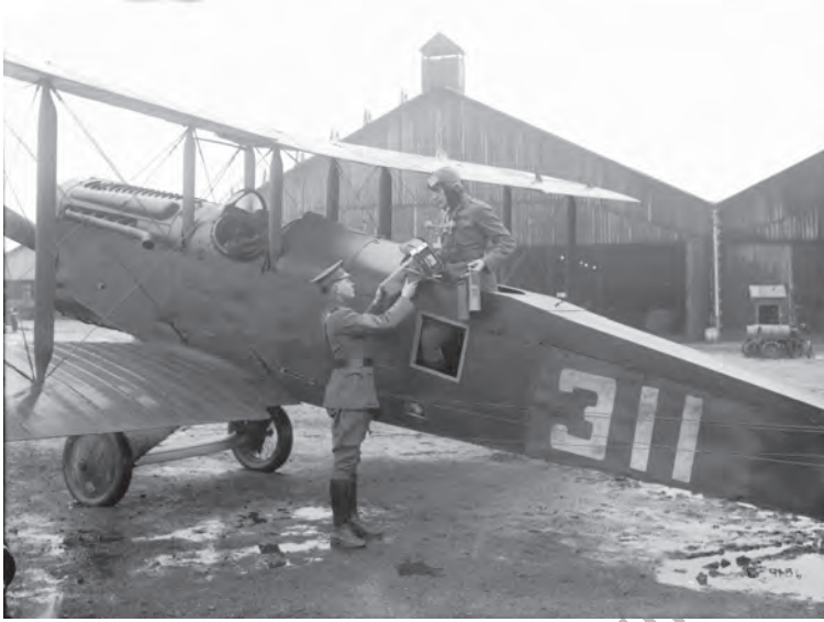
FIGURE 1.3. Aerial photography, World War I. By the time of World War I, attempts to match the camera and the airplane had progressed only to a modest extent, as illustrated by this example. The aircraft (with the biplane design typical of this era) has a port for oblique photography to allow the photographer to aim the camera through the port from within the fuselage to avoid the disadvantages of leaning over the edge of the cockpit. The photographer wears a chest-mounted microphone for communication with the pilot and is shown holding a supply of extra plates for the camera. From U.S. National Archives and Records Administration, Still Pictures, E-4156.
