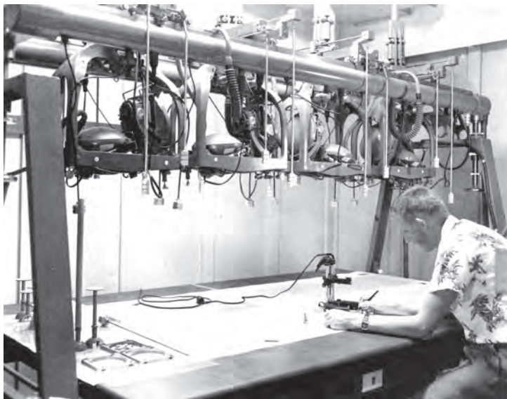
FIGURE 1.7. A stereoscopic plotting instrument used to derive accurate elevation data from aerial photography, 1957. During much of the twentieth century, photogrammetric analyses depended on optical–mechanical instruments such as the one shown here, designed to extract information by controlling the physical orientation of the photograph and optical projection of the image. By the end of the century, such processes were conducted in the digital domain using electronic instruments. From Photographic Library, U.S. Geological Survey, Denver, Colorado. Photo by E. F. Patterson, no. 223.
