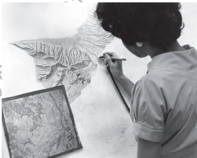
FIGURE 1.8. A cartographic technician uses an airbrush to depict relief, as interpreted from aerial photographs, 1961. Within a few decades, computer cartography and GIS could routinely create this effect by applying hill-shading algorithms to digital elevation models. From Photographic Library, U.S. Geological Survey, Denver, Colorado. Photo by E.F. Patterson, no. 1024.
